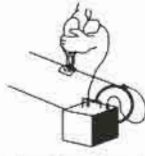
The cable and lug are brazed to the pipe
