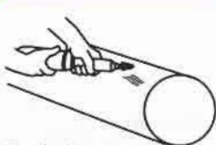
Clean the pipe
